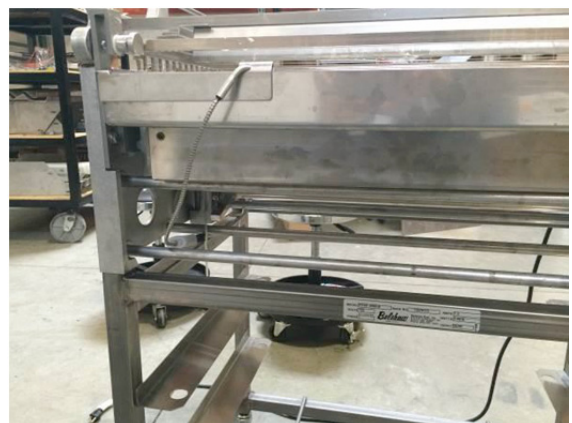
Figure 6, Installation of Thermocouple
