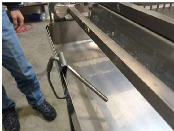
Figure 7, Installation of Thermocouple
