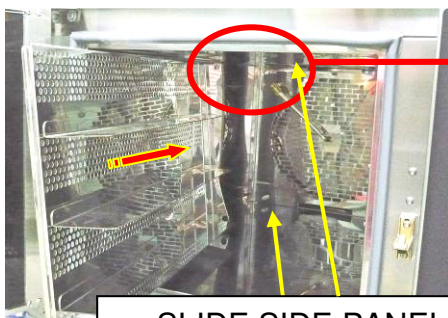
SLIDE SIDE PANEL OVER LOCATING PINS. TOP AND BOTTOM
