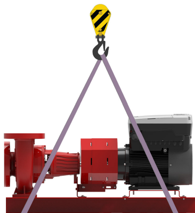
Acceptable lifting methods for base-mounted models e-1510X and e-1532X
