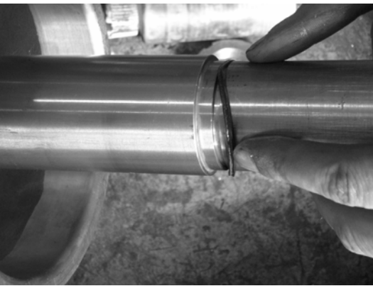
Figure 37: Installing the Quad Rings
