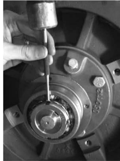
Figure 50: Installing the Lockwasher and Locknut
