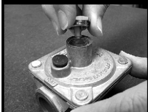
2. Locate the plastic part attached to the brass cap
