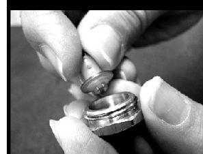
4. Snap the plastic part off of the brass cap
