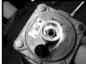
8. To adjust pressure: Remove brass cap & turn white plastic part inside the stem of regulator
