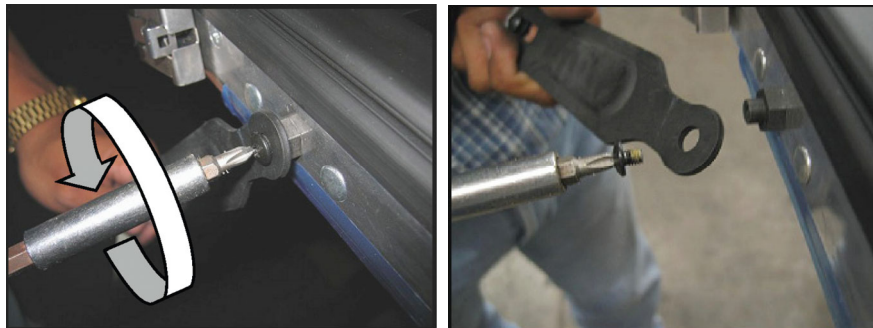
Figure 13.1 Removing hold-open assembly from door .
