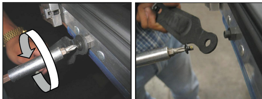
Figure 13.1 Removing hold-open assembly from door .
