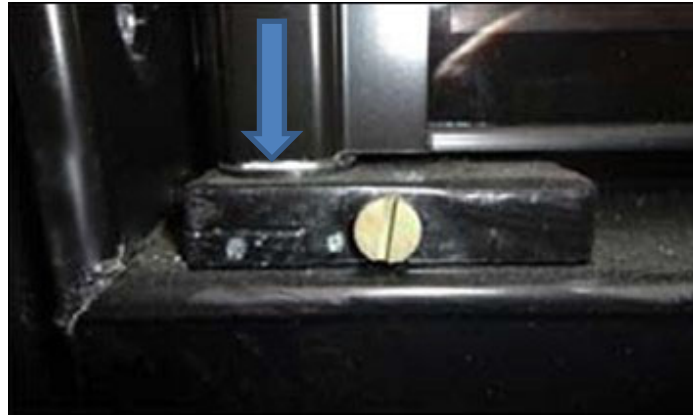
Figure 4.1: Seating Door onto Torque Master
