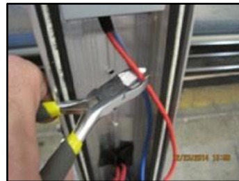
Cut wires at the bottom of the driver (red & blue)
