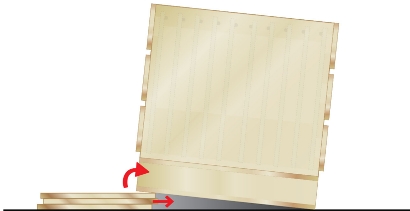
Figure 3.4. Offsetting crate weight for removing doors from the crate
