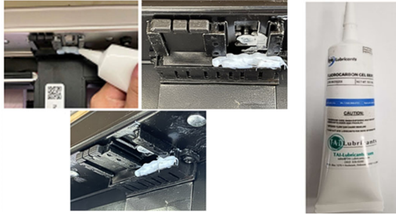
Figure 17.2: Dielectric Grease in SOCKET (hinge pin plug) receptacle
