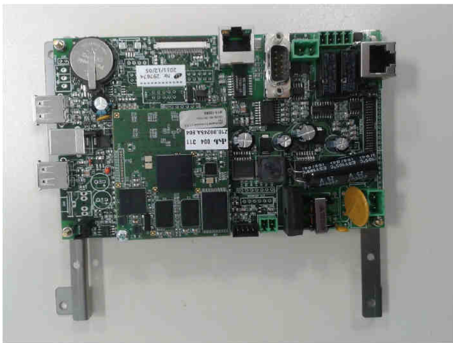
CPU board mounted with KIT
