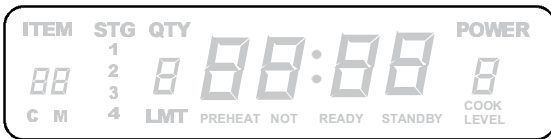
OFF condition Initial Power-Up
