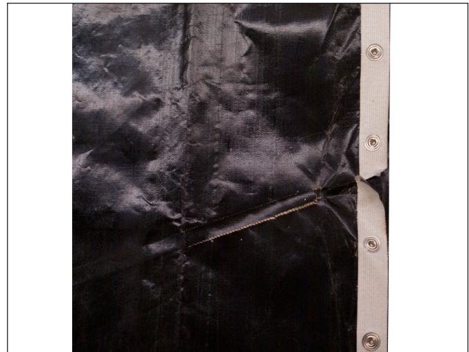
BELT IS MISSING SNAPS AND IS DAMAGED. REPLACE BELT.
