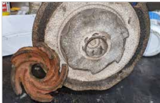
Impeller damaged from high acid solution
