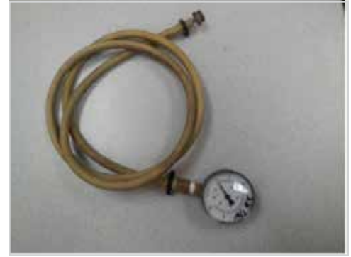
Spray arm pressure tester #088-1048
